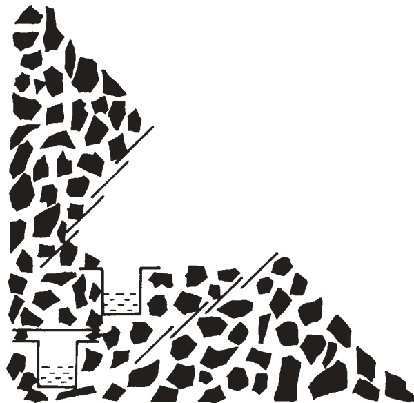
Fig. 3. Cross-section through an probe inserted in the scree slopes. Telescopic metal rings share up the sides of the hollow in the scree, in which pitfall traps with preserving fluid, and a roof are installed.
